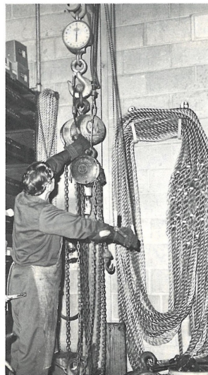
Expert in the care of rigging equipment is Lynn Cochran. Eying the gauge, Lynn tests a chain hoist in the tool repair area.
