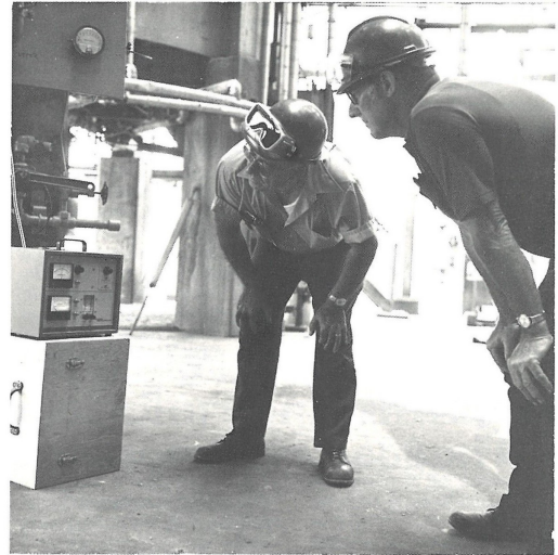
Bill Klockenga (left) and Joe Lanzerotte watch as the needle measuring oxygen content in an Aromatics furnace drops as a result of air intake adjustments. Similar exercises are carried out daily in other operating departments.
