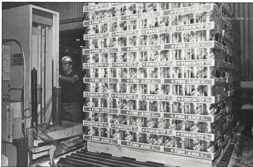
A pallet of tray-packs is enclosed with a protective layer of plastic at the stretch wrap machine while Rich Carmean, machinist, makes mechanical adjustments. After wrapping, the pallet is moved into the PLW for storage and shipment to a Shell customer.
