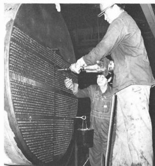
"Rolling the tubes." Using a special tool, Frank Carrigan expands the outer couple inches of each tube to assure a tight fit. Leon Little applies oil to reduce friction. Both are boilermakers.
