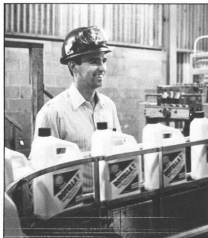
Dave Hutton, project engineer for the gallon bottle line, smiles as he watches the new system fill and package Rotella T gallon jugs at a rate of 90 gallons per minute.
