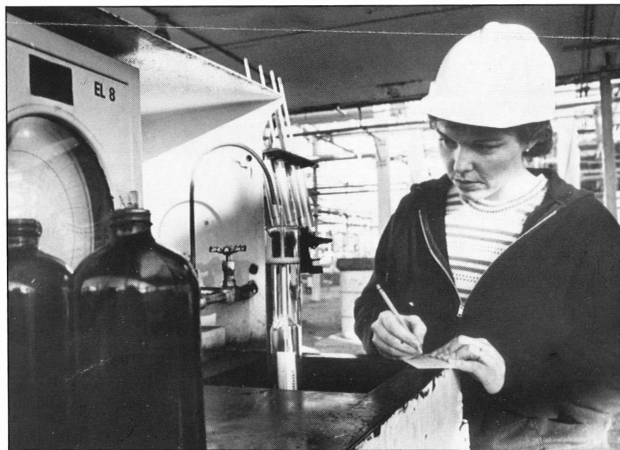
Karen Werner , a Shell Pipe Line operator in Wood River, tests a sample of jet fuel for quality before the product is sent by pipeline to Shell Distribution Plants in the midwest.
