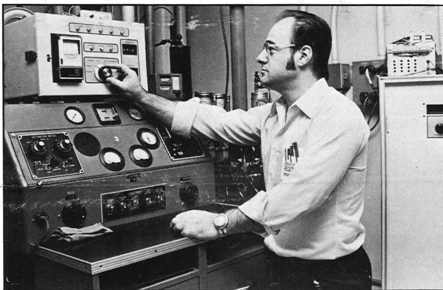
Bill Gray, Motor Lab operations foreman, adjusts one of WRMC's new octane engine controllers. The partially installed computerized system was designed by Shell's Westhollow Research Center, Houston.
