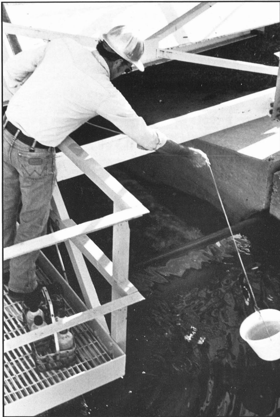
Leroy Edwards, Utilities, collects a sample of water before it enters the Mississippi at the lagoon outfall. Water used by the Complex in the refining process is treated before it is released into the river.
