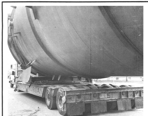
REALLY BIG MOVE. This giant flatbed with 24 tires was able to accommodate only about half of a 75-ton, 84-foot asphalt converter vessel moved from Shell's docks through Hartford to the refinery. A special dolly with 16 tires held up the rear. For a picture story of this unique move, see page four.
