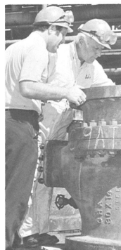
MAN-SIZED VALVE. Ron Banducci, Cat Cracking process manager, and Jim Becker, operations shutdown coordinator, inspect a huge slide valve to be installed during the shutdown.
