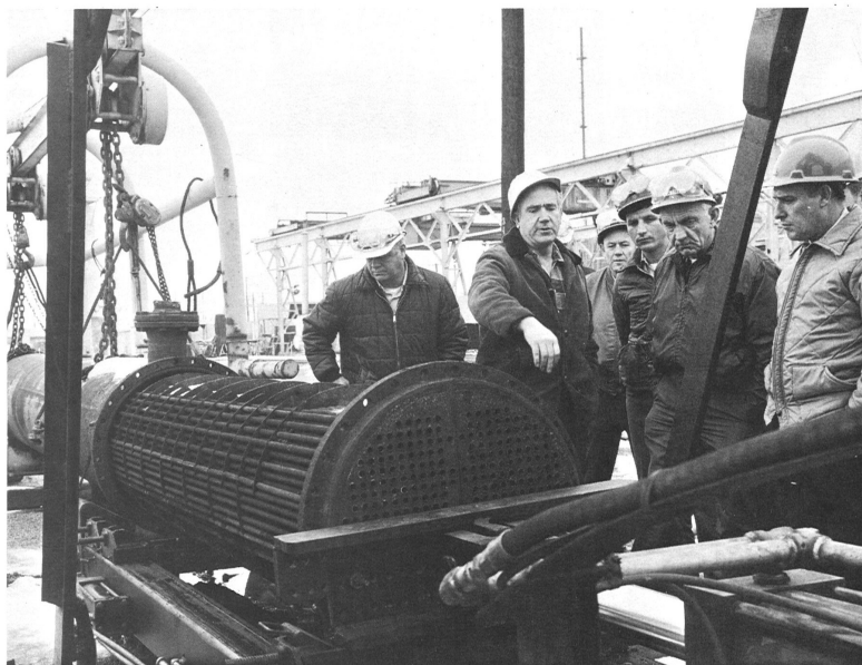
HERE'S HOW IT WORKS. Red Donaldson (second from left) demonstrates the potential capabilities of the new hydraulic bundle extractor.
