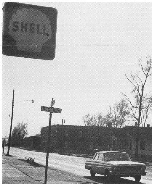
ONE OF TWENTY-FOUR Ford Falcons in Wood River Research Laboratory's test fleet is shown here on Central Avenue in Roxana on one of its short four mile trips at low speed. The cars, driven four miles once every four hours or more, are operated under simulated city driving conditions at speeds under 35 miles per hour.
