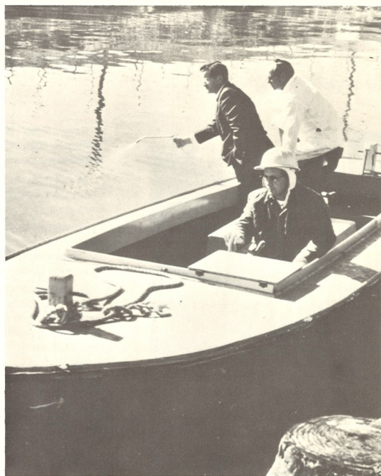
Because of the relatively low dosage rate required, when the On-Scene-Coordinator has agreed to the use of Shell Oil Herder -- only two gallons per linear mile of spill perimeter -- a common hand-operated garden spray may be used from a boat for small spills occurring in harbors, marinas, lakes and inland waterways.
