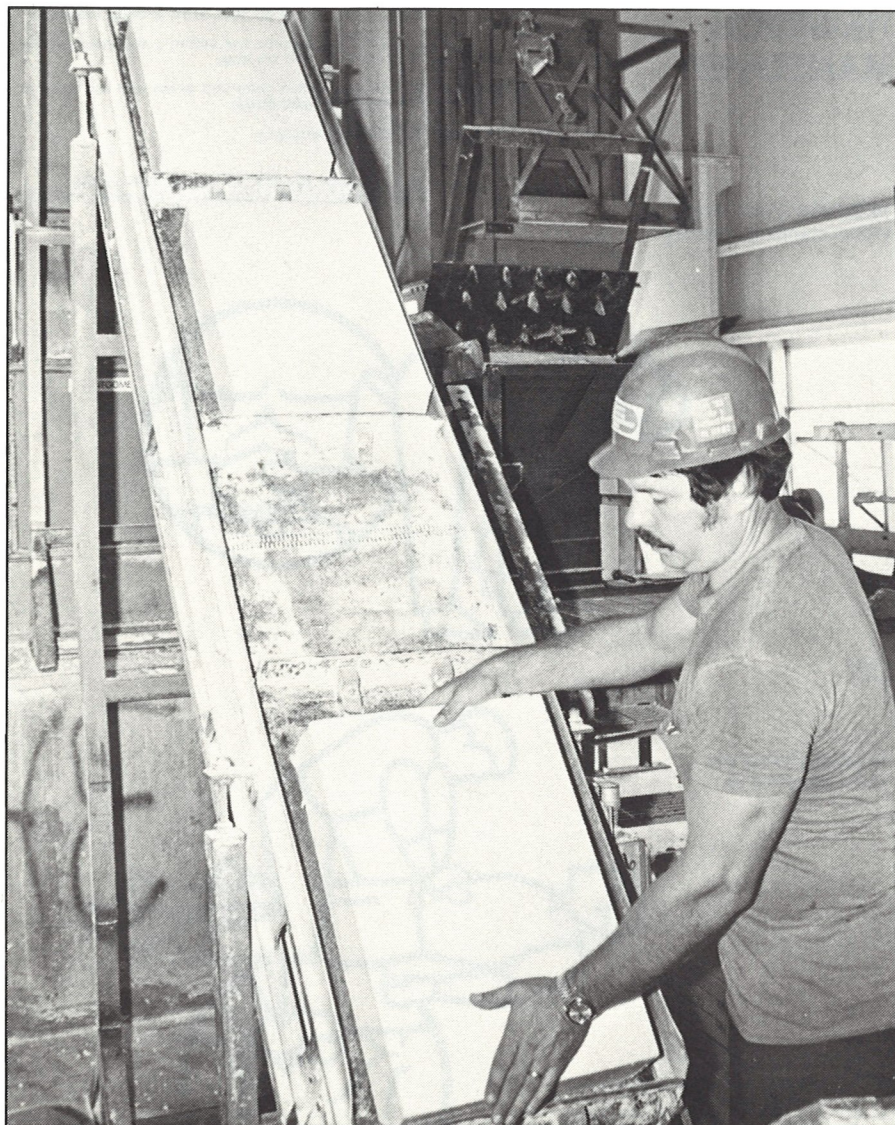
Dave Bristol, WRMC Compounding, loads bales of Shellvis® onto a conveyor that feeds a chopping machine. The bales are ground into granules and dissolved in base stock oil to make Shellvis concentrate which is an important multigrade motor oil additive. The Shellvis is produced at the Marietta Chemical Plant, Ohio.
