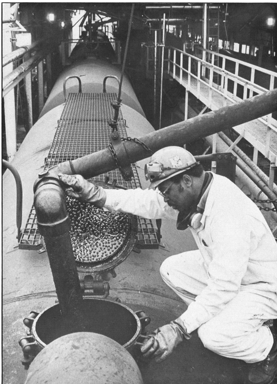
Ed Young loads a rail tank car with asphalt. During the summer peak season, the Complex can fill approximately 400 tank cars a month for shipment to customers in the Midwest and South.
