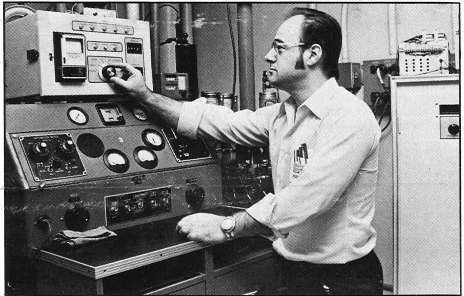
Bill Gray, Motor Lab operations foreman, adjusts one of WRMC's new octane engine controllers. The partially installed computerized system was designed by Shell's Westhollow Research Center, Houston.
