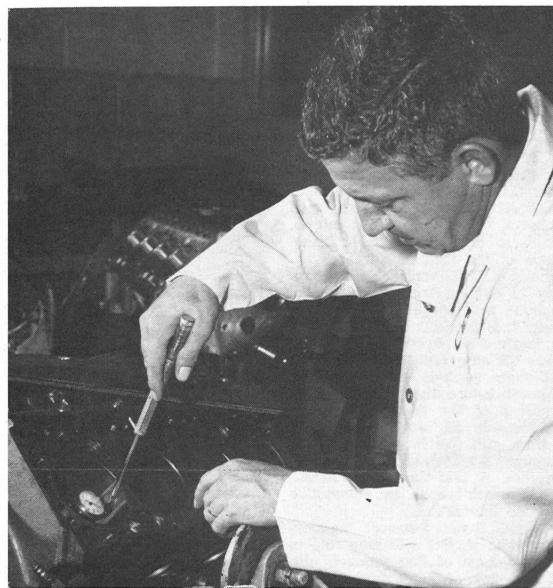
MEASURING WEAR in engines in which the new oil was tested was one of the many important examinations made after tests. In this photograph, Research Mechanic M. C. Franich measures for cylinder wall wear in an Oldsmobile engine after a test is completed.
